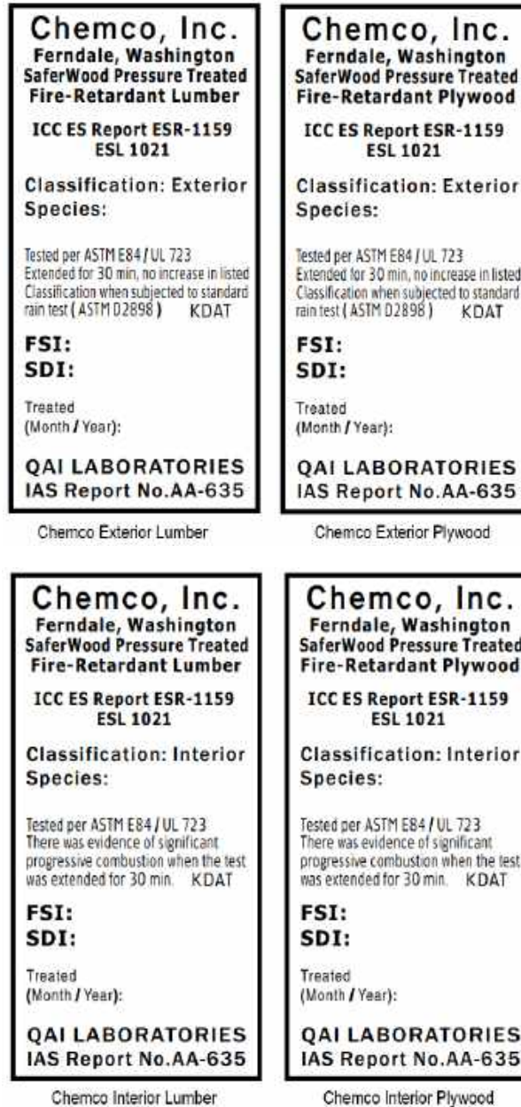
FIGURE 1—TYPICAL LABELS FOR FRX, SAFERWOOD-FX, THERMEX-FR AND MATAVERDE FIRE-RETARDANT LUMBER AND PLYWOOD
